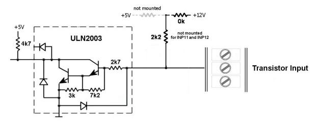
Note: 2.2kOm resistor mounted for INP1...INP10 only, INP11, INP12 without pull-up resistors
